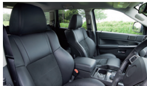
Automobile seats with cushion materials made using propylene oxide as a raw material
