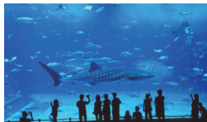
Large aquarium panel made of methyl methacrylate
